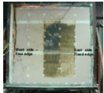
1. Unexposed face of test specimen after the completion of the test
